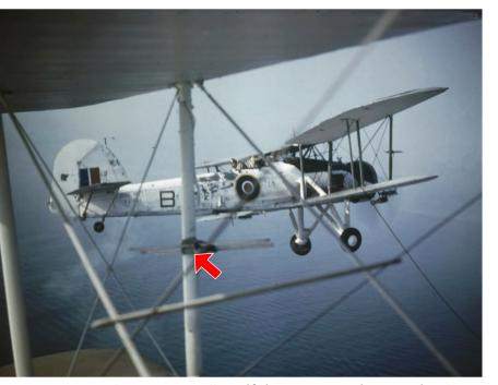
A war-weary Swordfish II on patrol. Note the Air to Surface Vessel (ASV) high gain "Yagi" radar antenna fixed to the strut in the foreground aircraft. Although rudimentary by today's standards, it was still capable of detecting a large ship at a range of up to 60 miles. It was less effective against the smaller U-boats but still played a pivotal role in the Battle of the Atlantic, including thwarting many attack opportunities. (IWM).
